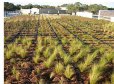
FIG 18: GREENGRID® is a Modular Green Roof System for Retrofit Applications
